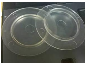
Fig.1. PLA monitoring caps for composite slab.
